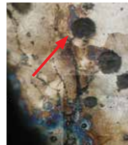
FerryNod® : crack is arrested/absorbed by graphite nodules
